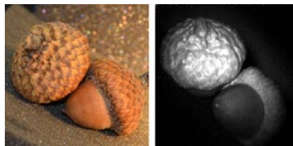
Figure 2: Image of the test objects taken with a DSLR camera (left) and a full-resolution reconstruction using the CS setup (right).
